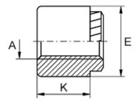
Female thread A = M3 Height K = 6 Hole diameter +0.1 = 4.2 Min distance to edge = 2.4 Min material thickness = 1.5 Outer diameter E = 7
